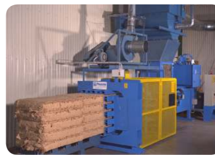
Compaction unit (baler)
